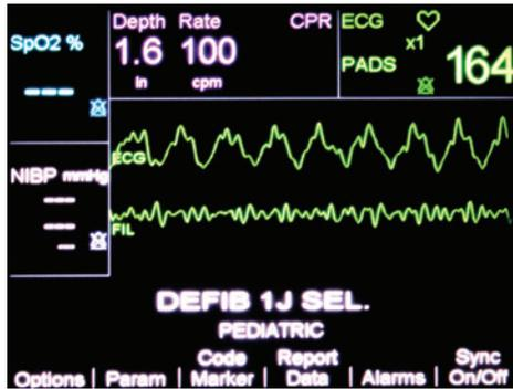
Figure 2. Display showing filtered and unfiltered waveform. (See-Thru CPR)
