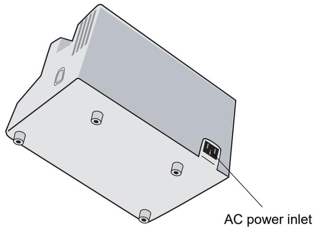
**Figure 2-2** *SurePower Single Bay Charger Bottom View*
