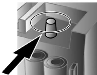
**Figure 1-3 Battery Key**
