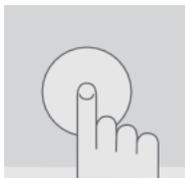
**Test** button. Pressing this button initiates a manual test of the battery.
