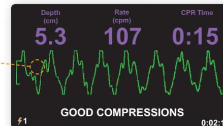
The AED 3 BLS can be easily configured to show the CPR Dashboard™ only, or both the CPR Dashboard and ECG. Depth and Rate indicators are highlighted in red if the compression rate is too slow and/or the depth is too shallow when in adult rescue mode.
